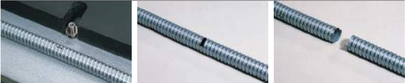
Corte longitudinal a través 2 espirales Cut longitudinally across 2 hose covering segments
